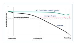
Bioplastics made from renewable raw materials conserve fossil resources and reduce greenhouse gas emissions. However, undesirable hydrolytic degradation often stands in the way of their use in technical applications. Employees of the Fraunhofer CCPE are therefore investigating various plastic additives in order to modify the service life of bioplastics and expand their range of applications.
